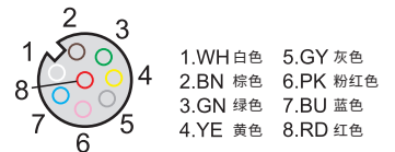
8针M12预铸电缆 8 pins M12 pre-moulding Cable
